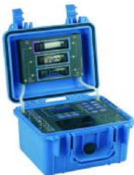
Figure 6.3 Analyzer for flue gas
