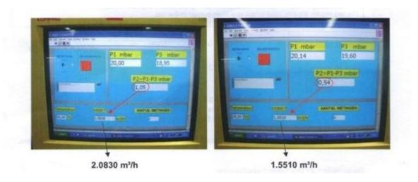
Test done with air at 20 m/bar at the inlet of the sample, the maximum flow possible with a pressure loss 0,5 m/bar, is 1,55 mc/h.
